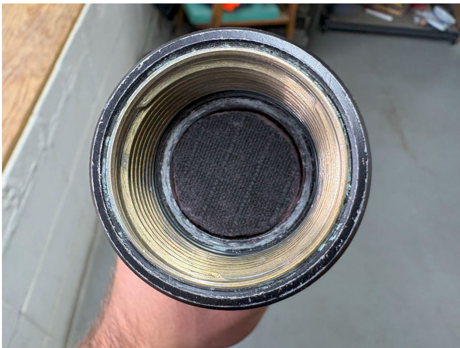
Figure 4 – Typical sample mounting for 29 mm diameter impedance tube
